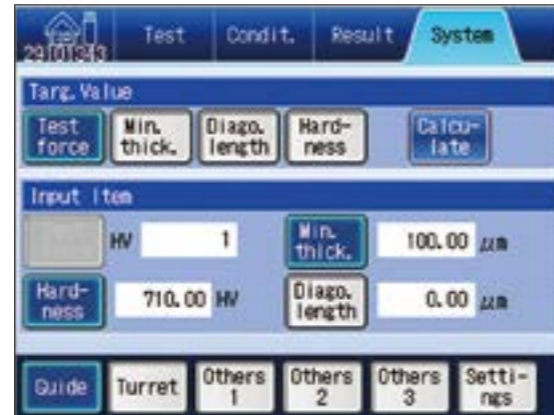
This screen supports setting of test conditions such as verification of the minimum thickness of a workpiece at the specified test force.
