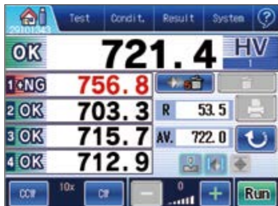
The list screen displays the last five test results, average, and variation. This screen is optimal for displaying the average of multiple test points.
