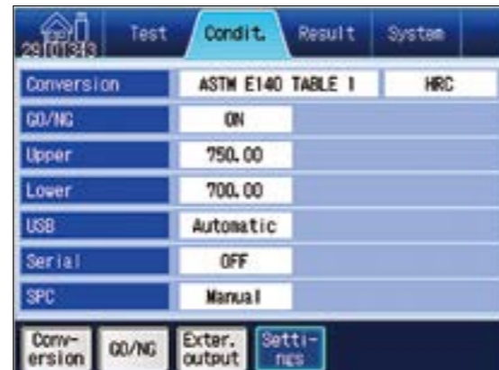
This screen allows setting of a conversion scale, GO/NG judgment and external output. It allows instantaneous verification of settings in the form of a list.
