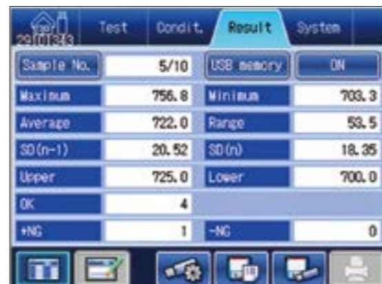
This screen provides a list of statistics of test results. It allows easy storing and printing results simply by clicking the icon.
