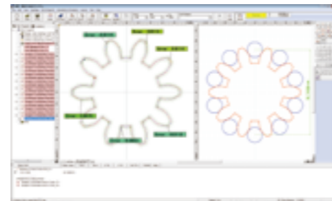
Example of gear contour matching, and an over-pin diameter analysis
