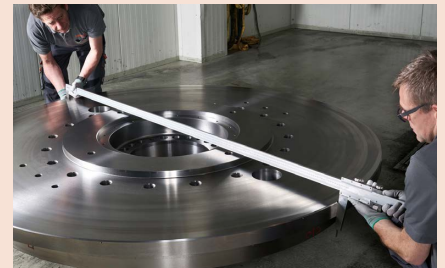
Radiused jaws for accurate ID measurement
